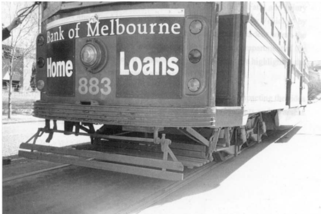
FIGURE 2 'W' class tram (17.7 tonnes) showing steel bumper height and under run frame.
