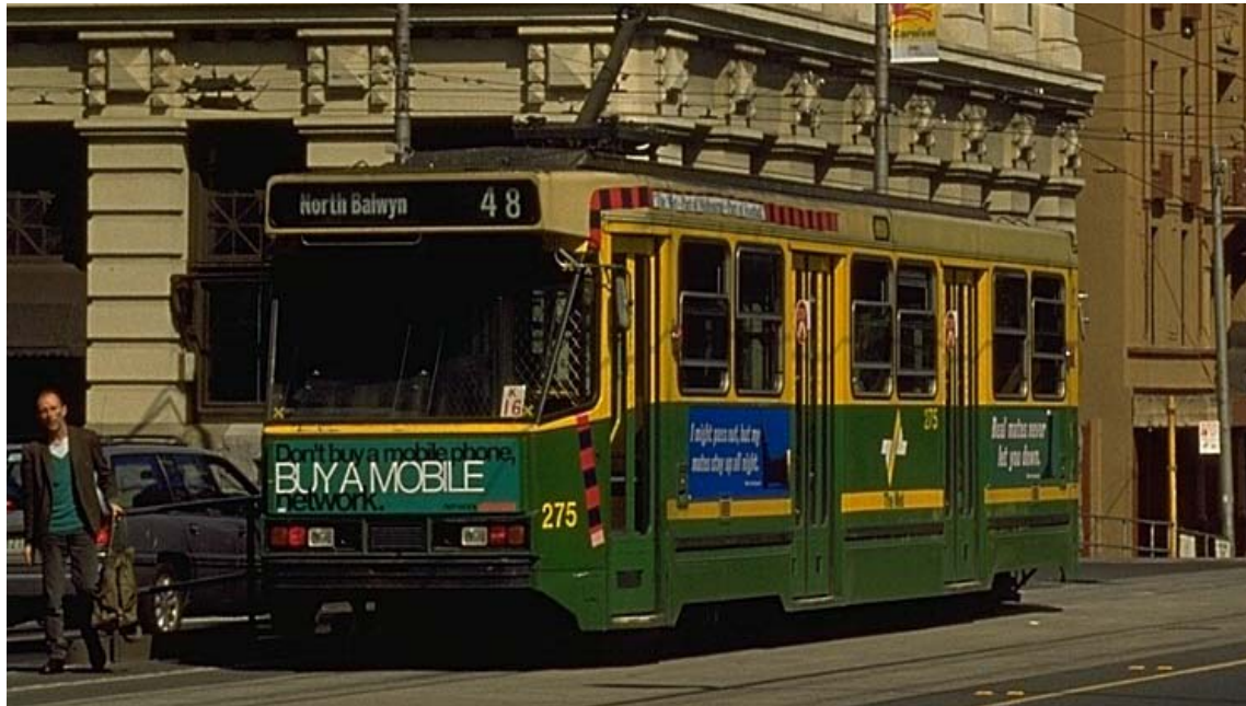
FIGURE 1 Close-up of steel bumper bar and under run gap below bar on 'A' class tram (22 tonnes). Note pedestrian safety zone between car and tram. (Photo by Clive Mottram from Geocities web site).
