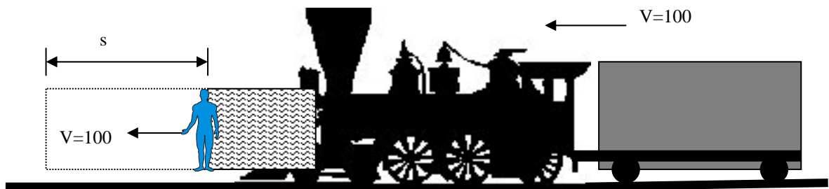
Figure 2b, impact between pedestrian and train with front airbag, after impact and deceleration distance 's'.
