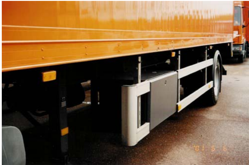
Figure 7. Side skirting to help prevent under-run in car collisions and over-ride of cyclists and motorcyclists during turning manoeuvres.
