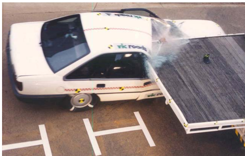
Figure 4. Under-run crash test between car and rear of truck.
