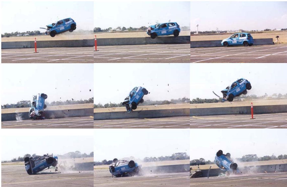
Figure 10. Small car impact into a concrete barrier at 80 km/h at 45 degrees.
