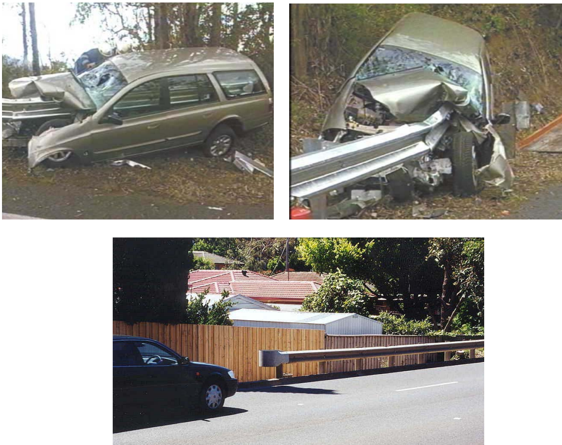
Figure 9. Photo graphs showing how guardrail end terminals can present an extreme hazard if not designed appropriately.
