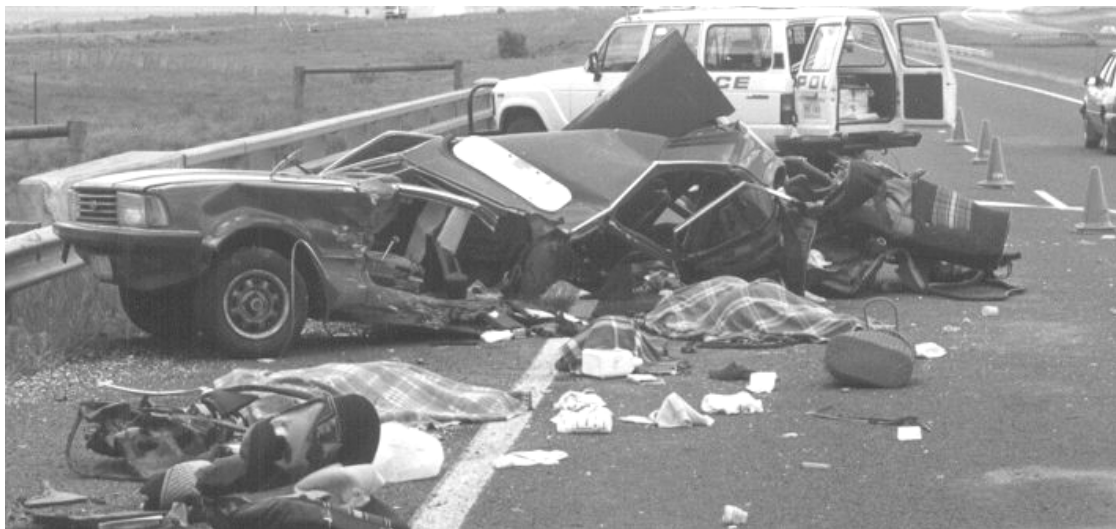
Figure 2. Extensively damaged vehicle, showing guardrail impact point near the front door.
