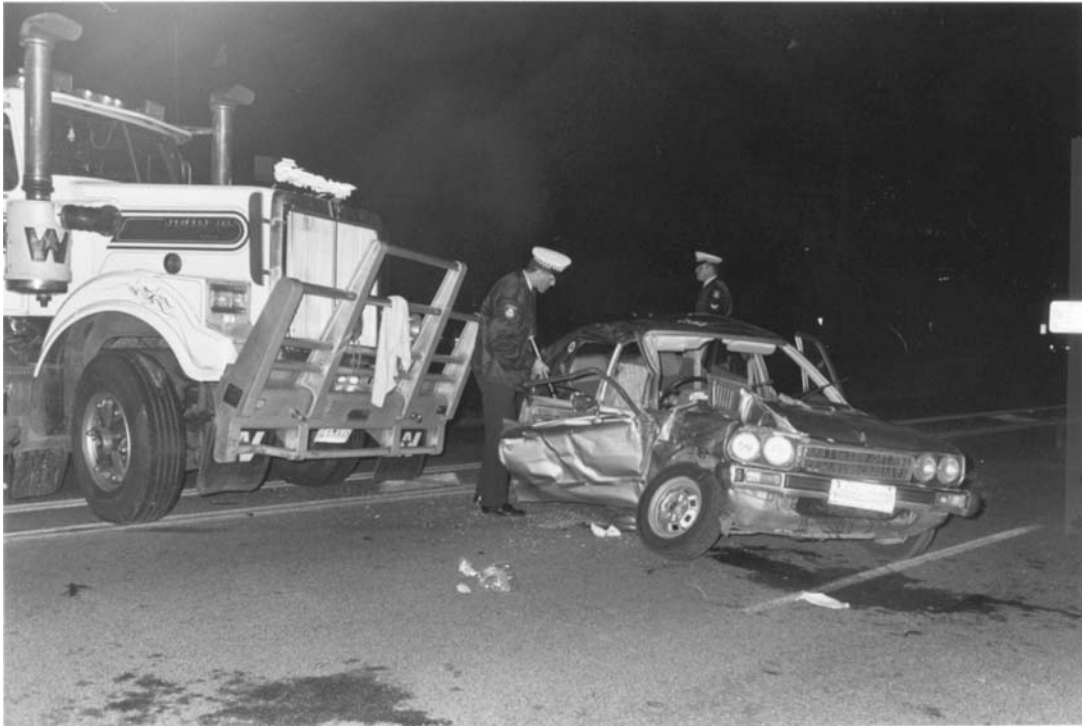
Figure 4. Crashworthiness incompatibility between heavy vehicles and other road users. Photo shows heavy vehicle crash with the side of car. Driver killed.
