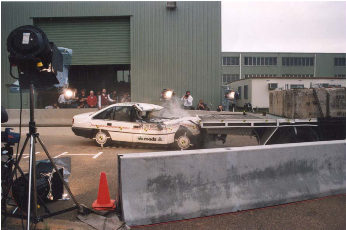
Figure 6. Under-run crash test at Monash University demonstrating incompatibility between car and rear of truck. Sketch on next page illustrates geometric incompatibility between the car and truck rear.
